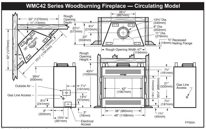
Fig. 2 WMC42 Series specifications and framing.
